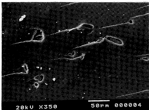
Fig.6A SEM photograph of 10 phr PC toughen epoxy.(350X)
