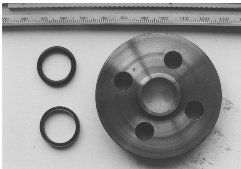
Fig. 6. The backup-ring and O-ring.
