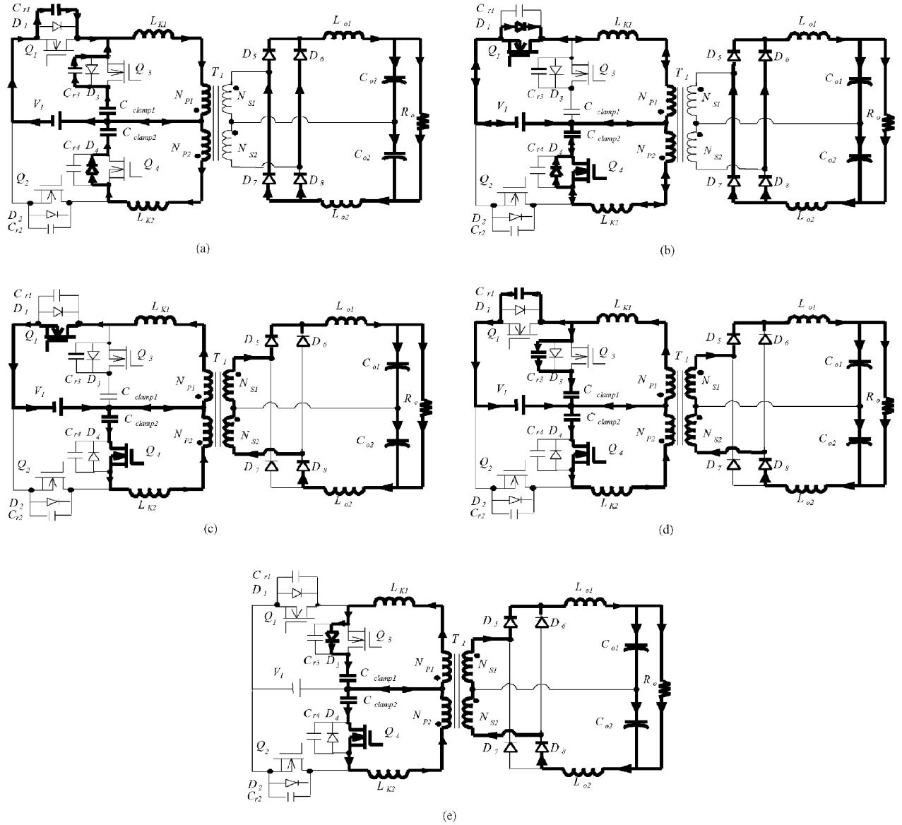
Fig. 3. Topological modes existing in the proposed converter operation over half a switching cycle.
