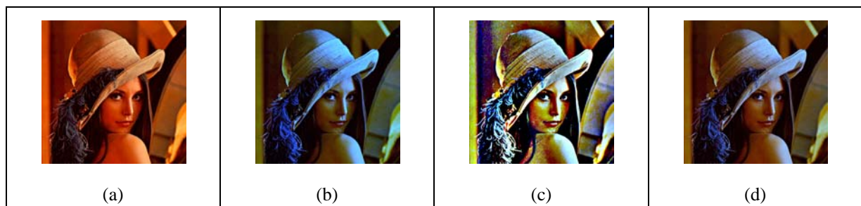
Figure 5 Adjusted results of an reddish image use the different automatic white balance methods: (a) original image (b) gray world assumption method (c) multi-scale retinex theory method (d) the proposed method
