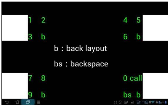
Figure 8. The GUI of mobile phone. Upper left square, upper right square, lower left square and lower right square indicates the flicker frequency of 5Hz, 7Hz, 9Hz, 11Hz, respectively.
