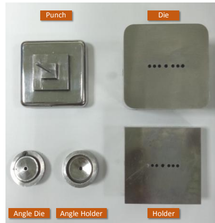
Fig. 3. Solid parts of the die.
