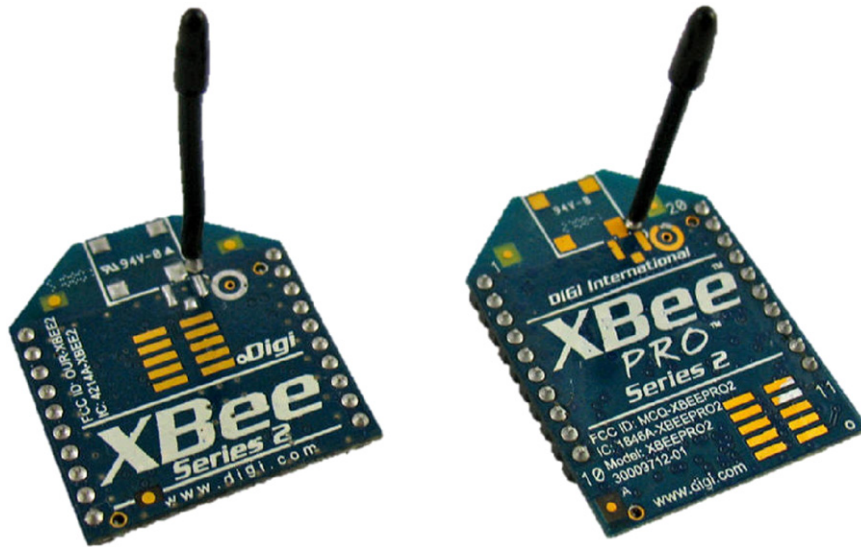
Fig. 4. XBee device in regular and PRO type.
