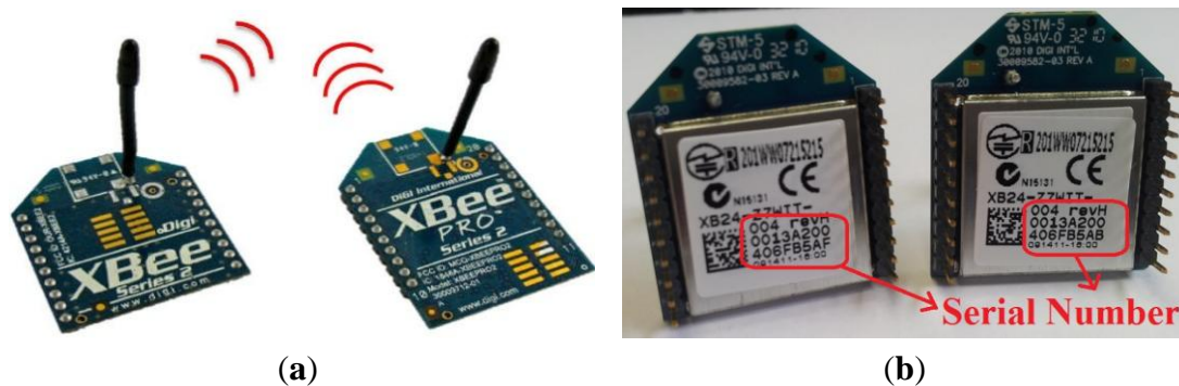
Figure 4. ZigBee modules. (a) Antenna on top; (b) Network hardware ID on the chip.
