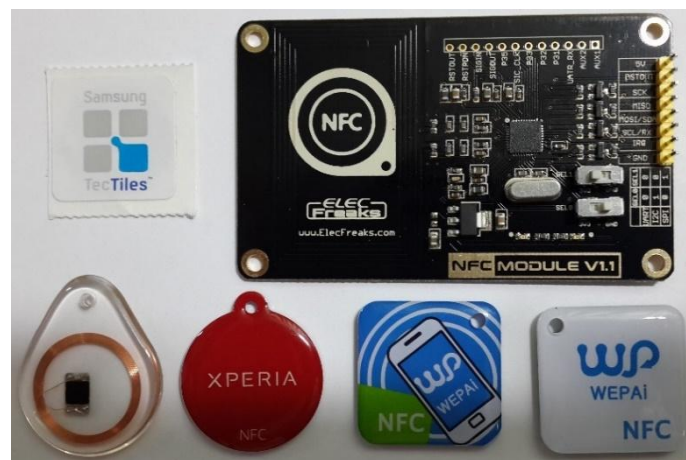
Figure 30. Relevant data or configuration written to a tag using NFC hardware module.
