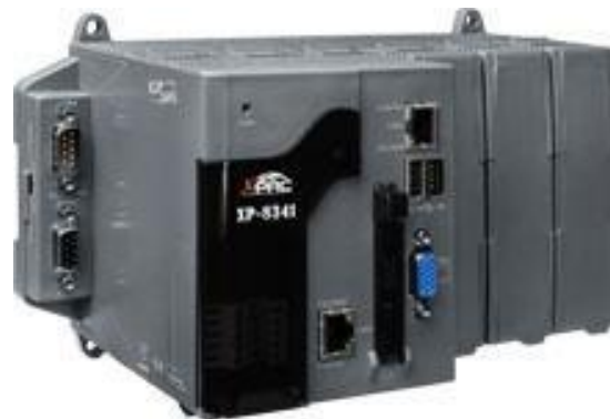
Figure 5. Photo of an XP-8000 controller as a server.
