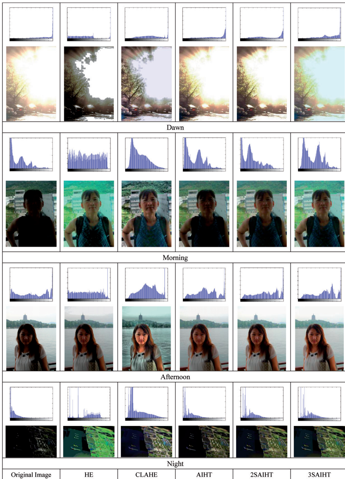
Figure 8. Various types of bad contrast images illustrating the difference between contrast enhancement by HE, CLAHE, AIHT, 2SAIHT, and our method of 3SAIHT.
