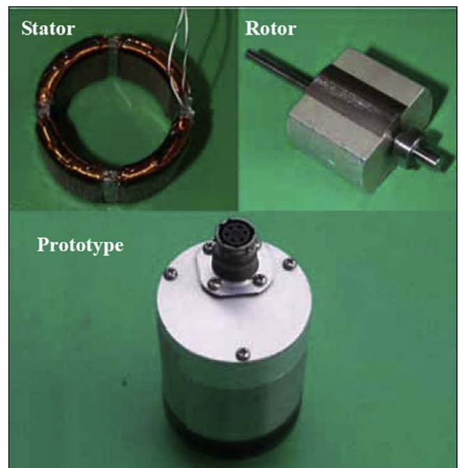
Fig. 5. Pictures of the designed stator, rotor and torque motor.
