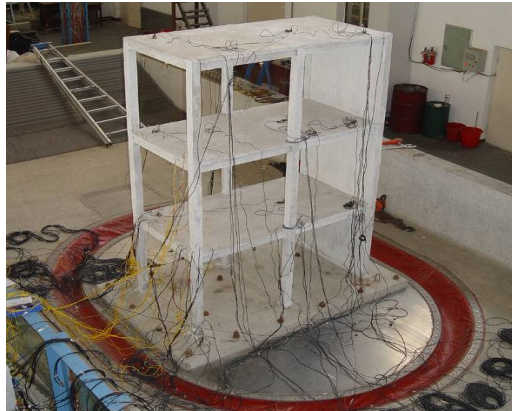
Fig. 3. Experimental setup for shaking table tests
