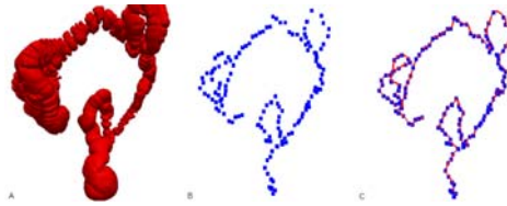
Fig. 6. In B are visible calculated key points, interpolated in C using a B-Spline
