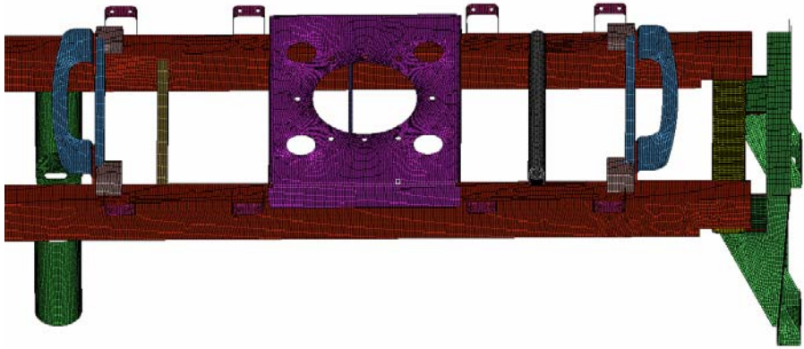
Fig. 2. Finite element model of the twin seat underframe
