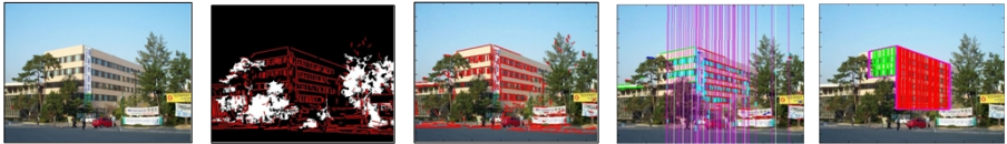
Fig. 3. The result of building detection: (a) original images (b) line segments detection and trees region (c) survived line segments reduction (d) dominant vanishing points detected by MSAC (e) mesh of basic parallelograms of face
