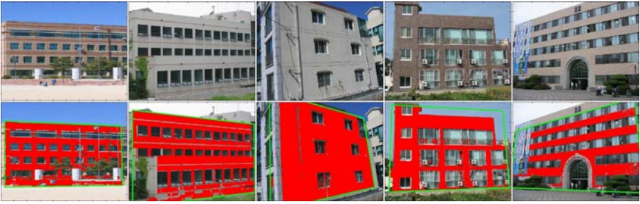
Fig. 2. Detection of building surface and wall region
