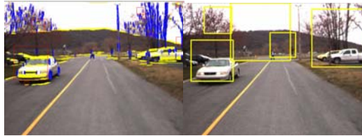
Fig. 4. Inaccuracy vehicle candidate regions(left) and right candidate regions (right) are detected
