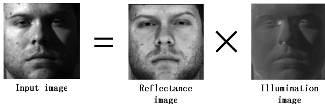
Fig. 1. The intrinsic images decomposition. The input image, from Yale B database, is decomposed into two parts, a reflectance image and an illumination image which are obtained according to [8].
