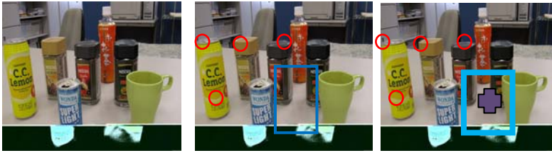
Fig. 10. Example of interaction by spatial relationships. The system tells the user that it knows the bottles (Coffee) and the can present. Then the user says that the target is in front of the rightmost bottle. The system detects the target indicated by “+” with purple.
