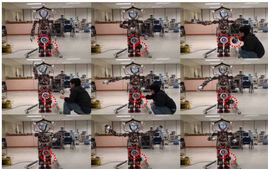
Fig. 12. Snap shots on the whole body motion and balancing test of humanoid robot under unknown disturbances, Dotted circles indicate the dumbbells employed as unknown disturbances
