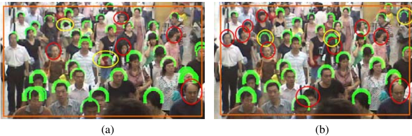
Fig. 4. (a) Results from our approach that directly matches on gradient map. Total pedestrians: 35, detected: 30, false alarm: 2, computing time in Matlab: 52s; (b) Results from the approach based on Canny Edge Detection and EDT. Total pedestrians: 35, detected: 25, false alarm: 3, computing time in Matlab: 108s. (Circles in the figures mark those undetected and false alarms.)
