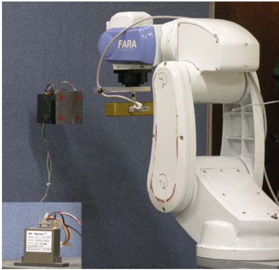
Fig. 6. Real-time experiment system configuration. Inside the object's box with landmarks on its face is the IMU. Object can move freely on four hanging threads.
