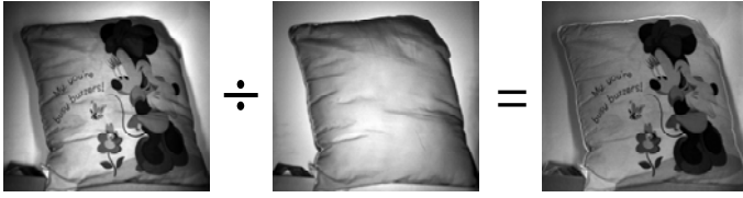
Fig. 6. The application of the proposed intrinsic image decomposition in object image processing. VIS image (left), NIR image (middle) and reflectance image (right).
