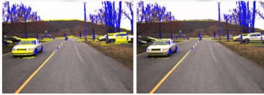
Fig. 3. Vertical and horizontal edges images (before and after repaired)
