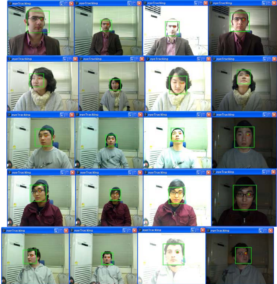
Fig. 4. Sample frames from sessions testing varying head positions, distance to camera and lighting conditions. The system still works accurately with shifted head position, test subject distance up to 1.5m, and exceedingly bright and dark environments.
