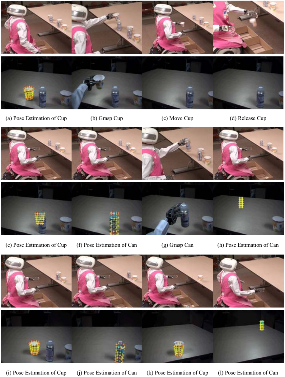
Fig. 8. The process of the task, “Classify Cups and Cans”. The upper images are from the exterior camera and the lower images are from the interior camera.
