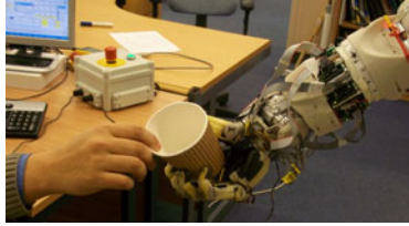
Fig. 2. The BERT2 anthropomorphic hand (right) during an object hand-over procedure
