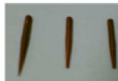
0.5mm 1mm 2mm 4 mm-in-diameter copper stick is lathed at one end to a 30
