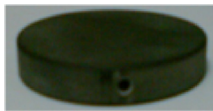
9 mm-in-thickness epoxy with a 3 mm-in-diameter cylindrical cavity
