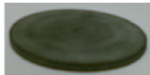
9 mm-in-thickness epoxy with a 3 mm-in-diameter cylindrical cavity
